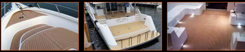
LONGEVITY - Built from planks of UV stabilised PVC. LOW MAINTENANCE - No regular wood sanding and oiling required, simply brush with soapy water. LIMITED DOWN TIME - One day to pattern, and one day to fit! All other work is conducted in our workshops. PRICE - Favourable pricing compared to real teak decking. QUALITY CRAFTSMANSHIP - High quality fabrication process of thermal welding to form deck panels. We do not glue planks together.
